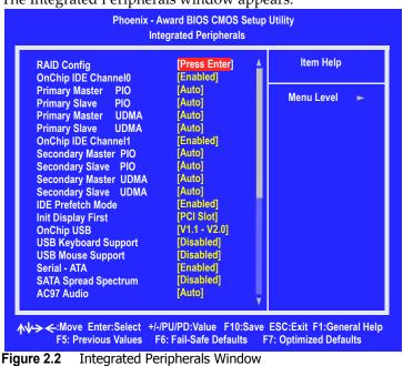
**3** Use the arrow keys to select the RAID Config (see Figure 2.2), then press Enter.
